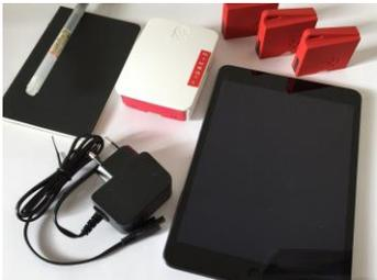
Figure 4: A probe pack with several sensors (SensorTags), a Raspberry Pi, an iPad, and a documentation booklet.
